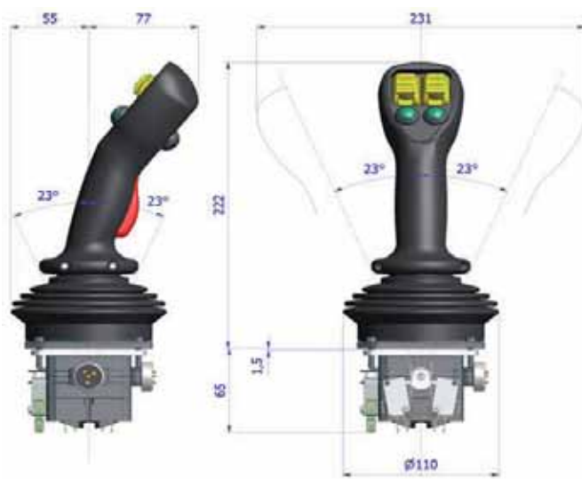
JMF base with MS type handle Complete code: JMF-L4C/NN-MS A2P9 2FPR R1P9
